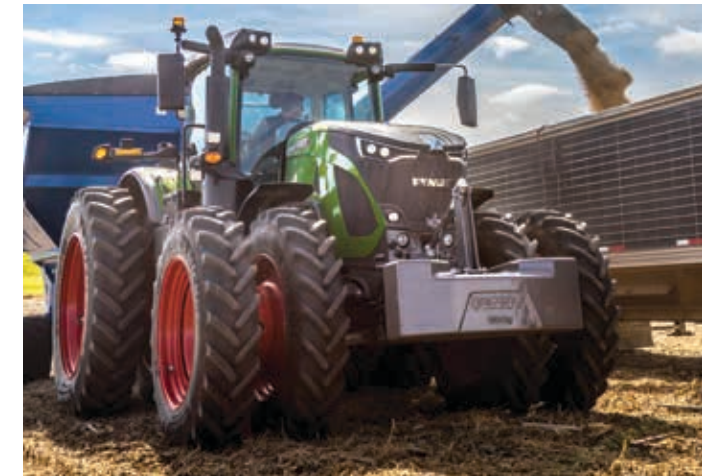
To ensure maximum power to the ground, the simple-to-adjust front and rear flexible ballasting system lets you increase the tractor's weight from 26,200 lbs. to a maximum ballast weight of 42,000 lbs.
