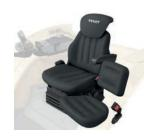
The comfort seat, with suspension and a mechanical lumbar support, offers excellent seating comfort. The instructor seat is cushioned and can be pivoted upwards to save space, if required.
