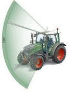
The built-in roof window provides an outstanding overview with an impressive 100° viewing angle. This gives you an unobstructed view, from the lifted front loader down to the wheel placement.
