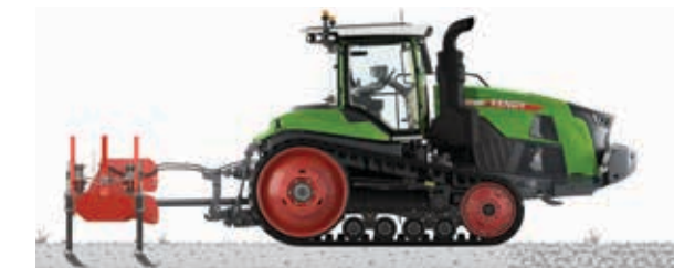
Figure 1: A tractor goes to work without proper tractor and implement weight distribution. This results in insufficient front weight on the tractor, and as a result increases slip.
