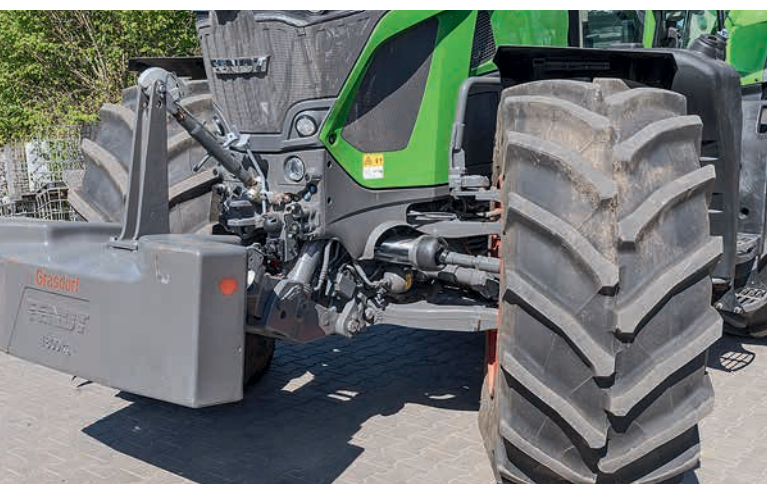
The front axle is permanently engaged at speeds up to 25km/hr.
