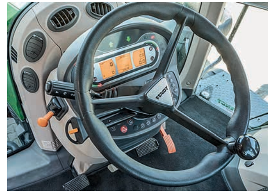
The dash replaces the A-post display. The handbrake lever is positioned a long way forward – luckily, it's not used too frequently thanks to the tractor's excellent parking lock.
