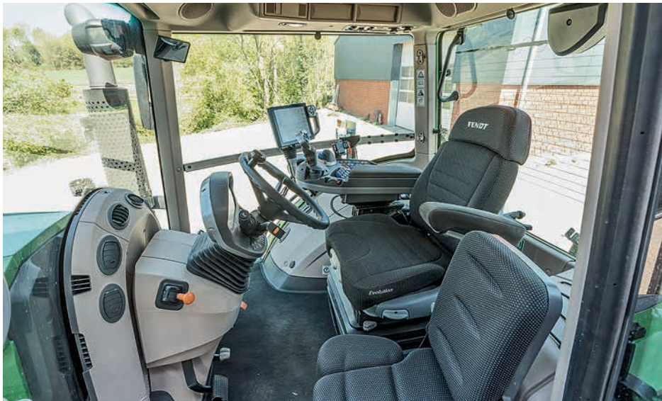
The accommodation is identical to what's on the 1000 series, but it's mounted on three suspension points.
