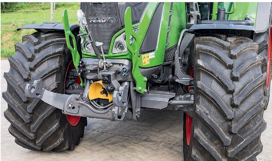
The front linkage has the option of a position control and dynamic relief. Front axle suspension is part of the standard package, but the front linkage (£3,408) and pto (£4,356) remain on the options list.
