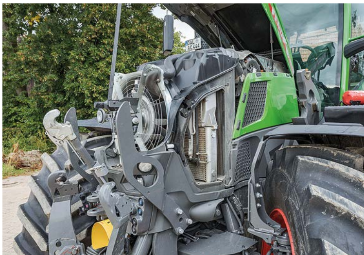
The air is forced through the cooling pack, and the 7.5-litre AgcoPower motor revs at a frugal 1,700rpm for an eyebrow raisingly low fuel consumption.
