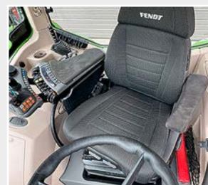
Small operator seat swivel range when looking behind.
