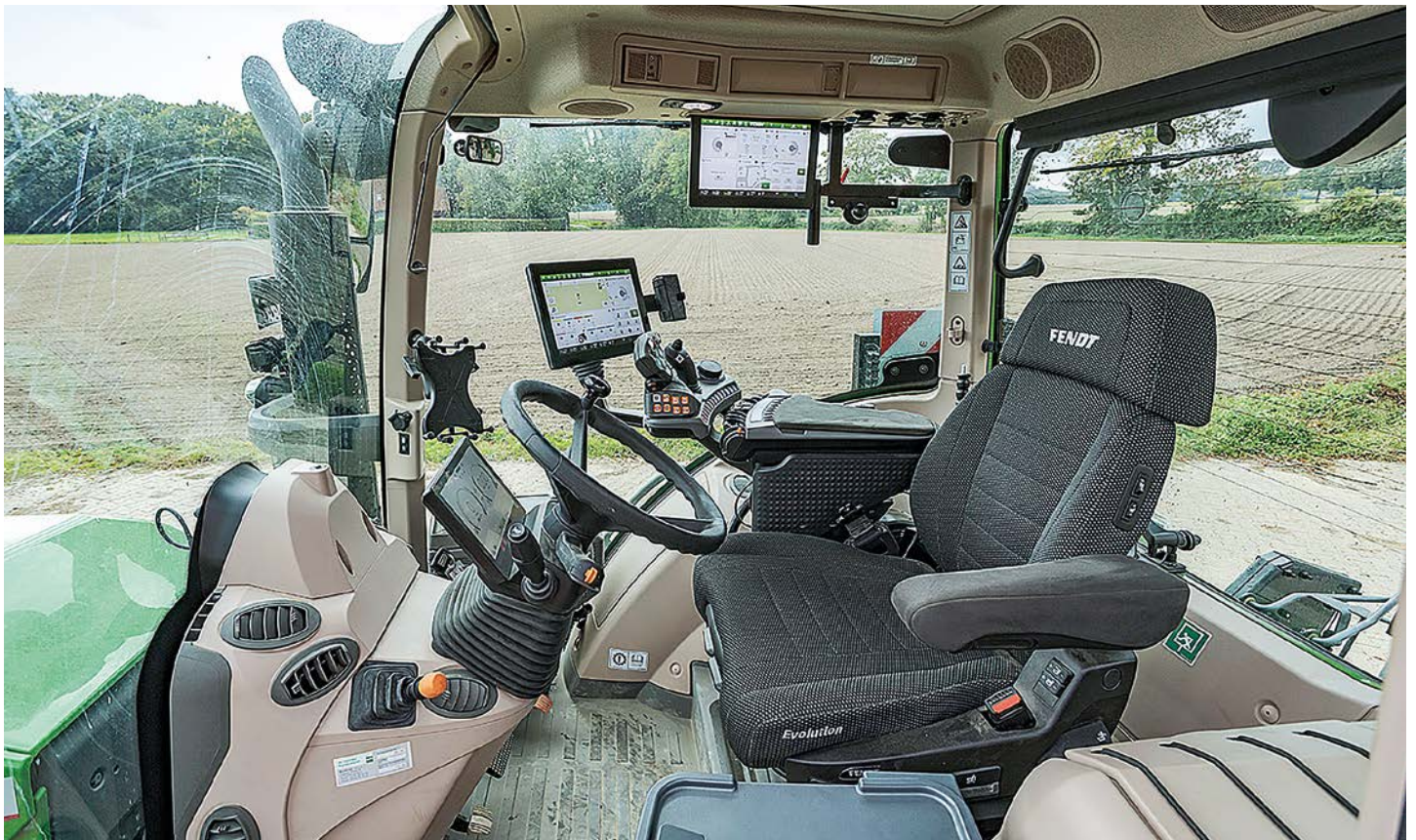
The cab is nice and quiet at just 69.5dB(A). Visibility is also good, albeit the sunblind and wiper motor do blot the view. And more space would be nice, too.
