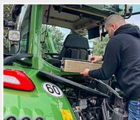
The cab filter is difficult to get at for cleaning/maintenance.
