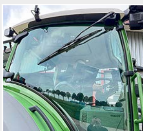
The wiper on the right window has a 97° wiper field.
