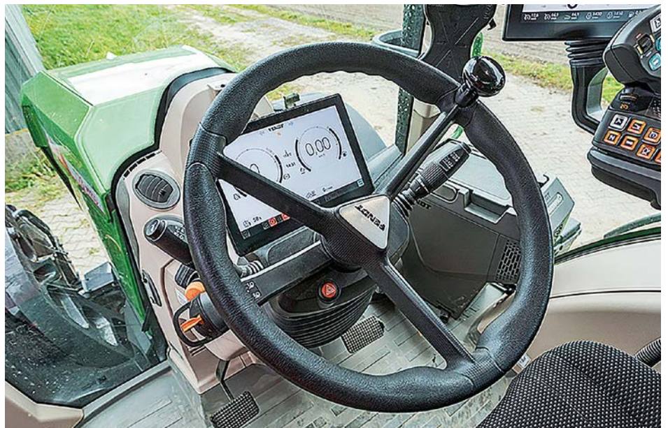
The spokes of the steering wheel interfere less with the display than we thought would be the case, although we still reckon the A-post mounted display used by competitors is a better solution.
