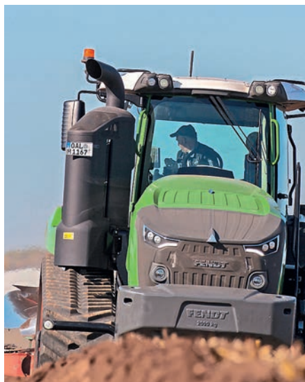
All of the tractor's Stage V exhaust emission gubbins (the DOC, DPF and SCR unit) are located in the huge stack on the right-hand side.
