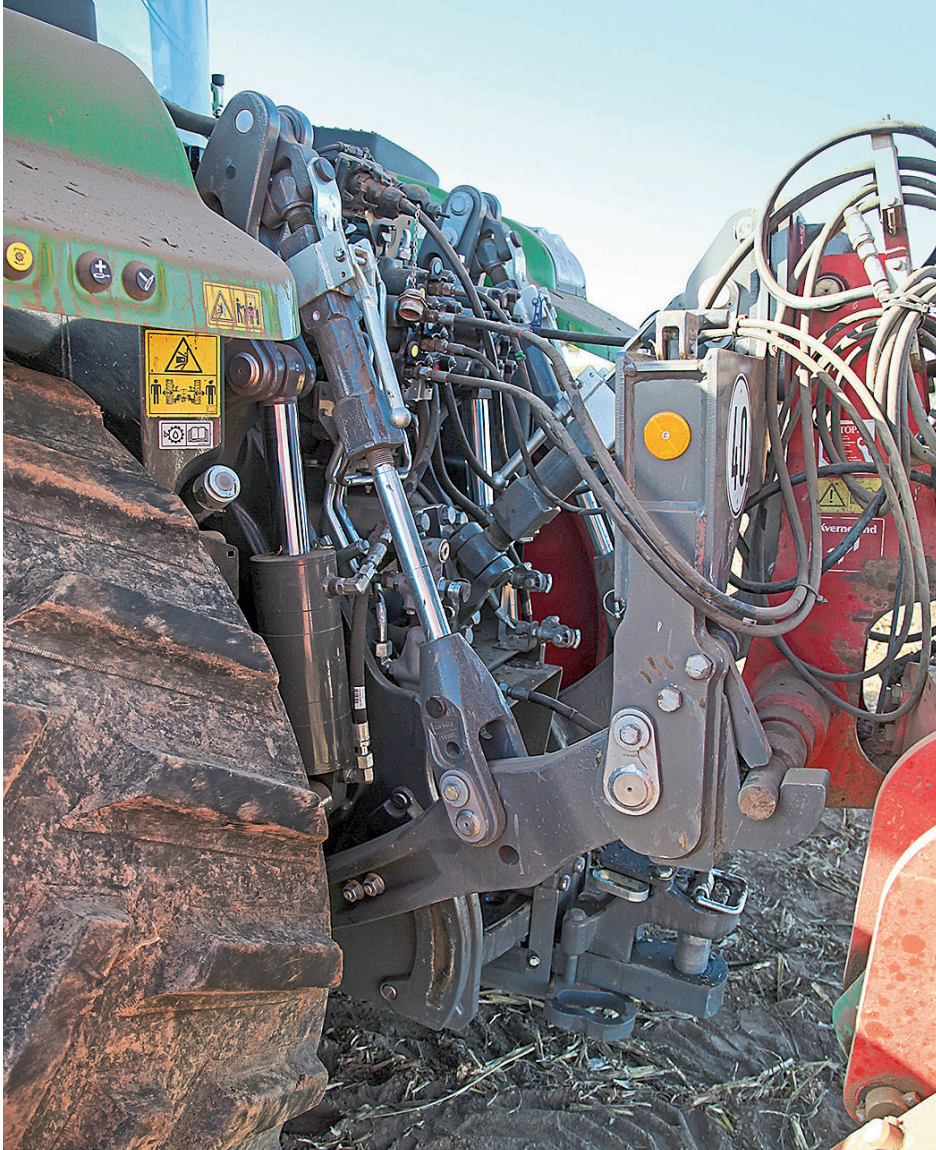
Neatly labelled connectors with relief levers – as they should be. Optionally up to eight double-acting spools and 440l/min oil flow are possible.
