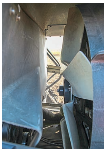
The six-cylinder MAN engine under a similarly large bonnet is both quiet and economical. The tractor's radiator pack is completely sealed off from the engine.
