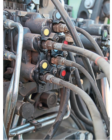
Neatly labelled connectors with relief levers – as they should be. Optionally up to eight double-acting spools and 440l/min oil flow are possible.
