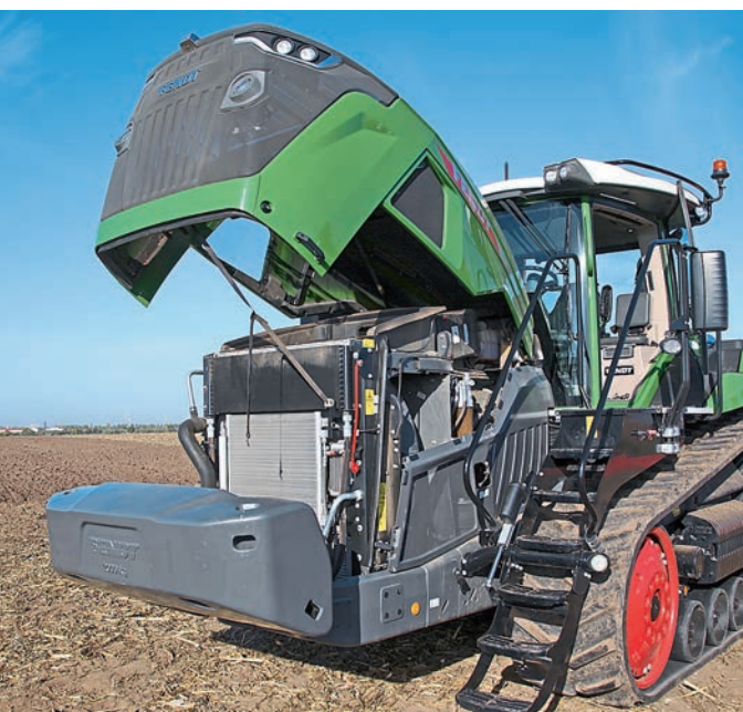
The six-cylinder MAN engine under a similarly large bonnet is both quiet and economical. The tractor's radiator pack is completely sealed off from the engine.
