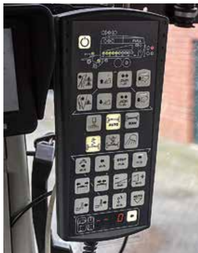
△ The actual machine functions were best operated from the Tigo control box.
