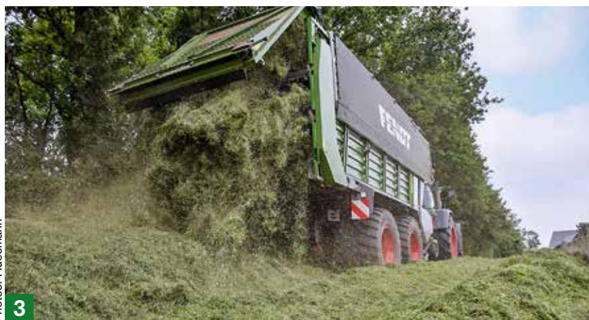
△ 1) The chain-and-slat floor slopes 25cm on a length of 1.60m towards the front. There are two pairs of chains with slats. 2) The quality of cut is good. The nominal cutting length is 37mm. 3) The two discharge rollers unloaded the material in a fluffy and uniform mat. A third roller is an option.
