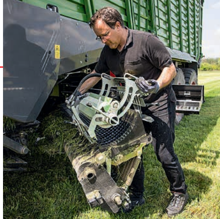
The blade sharpener is stored on the machine and placed on the knife back to freshen up 10 blades at a time.
