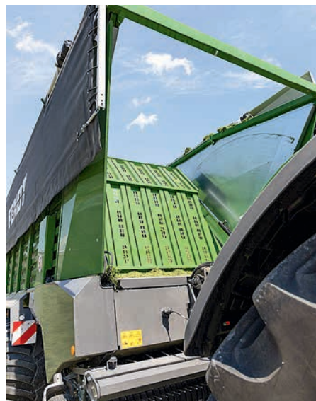
Pressure sensors in the rams for moving the headboard help control the loading process and pre-compression of the material being ingested.
