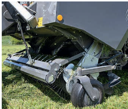
Ground contouring for the wagon's 2.20m wide pick-up is taken care of by gauge wheels on the sides and a roller at the rear.
