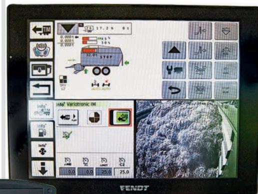
TIM is activated from the Vario-Terminal and kicks in when the cruise control is enabled.
