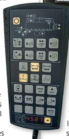
The wagon's functions can be operated via ISObus or in parallel with the pictured control box.
