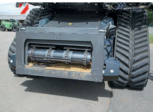
The feeder house measures a narrow 1.40m, but it has four chains that still pull through a decent volume. Our test machine unfortunately lacked the automatic header attachment system.
