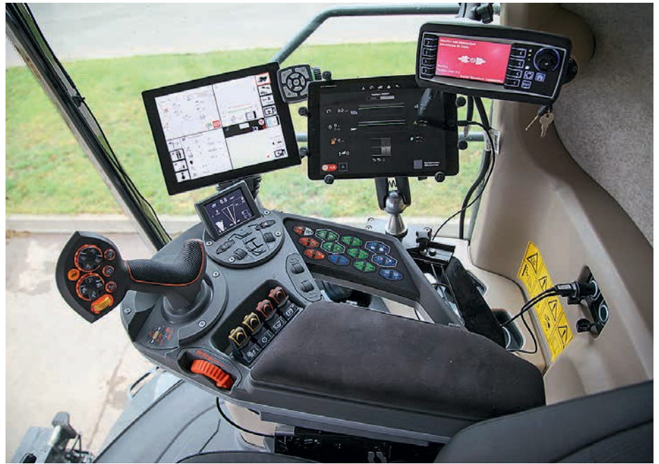
All controls are grouped neatly and logically, but a tablet is required to use IdealHarvest auto-adjustment. The Geringhoff header on our test combine was also operated via a separate terminal.
