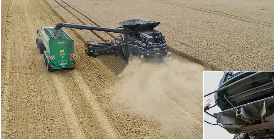
After a tweak to the way in which the ActiveSpread SwingFlow was installed, chopped straw was distributed evenly.
