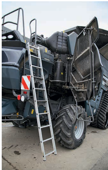
Access to the engine and 1,250-litre fuel tank are convenient. There is a 1,500-litre option.
