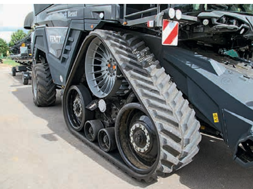
At 2.0m high and almost 2.0m long, the 76.5cm wide tracks keep machine dimensions below 3.5m. They are also suitable for 40 km/hr on-tarmac travel, but, surprisingly, drive power is in short supply on steep roads.
