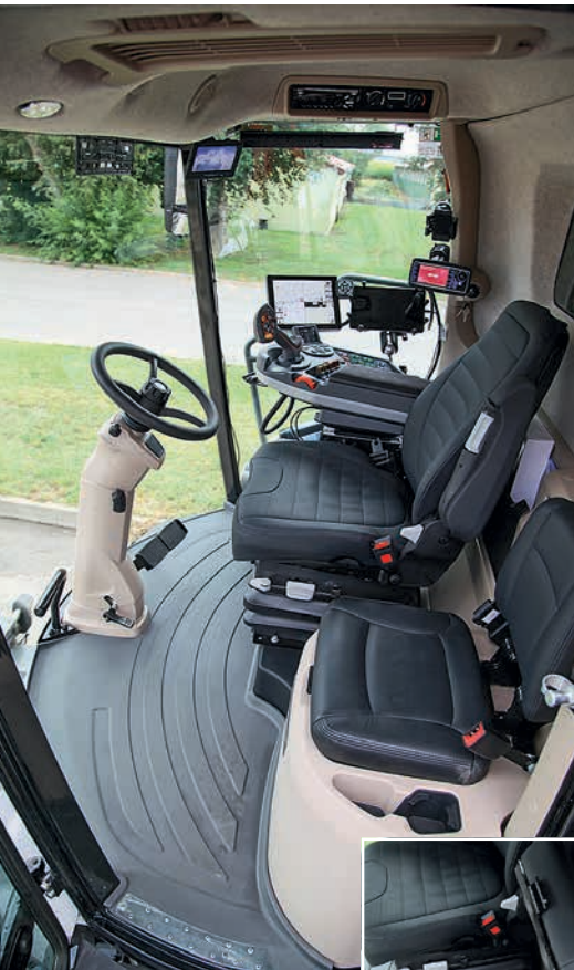
The cab is comfortably furnished, has a large cooling box, and noise levels are OK at 77dB(A). Our only gripe is with the Ideal's hands-free phone system.
