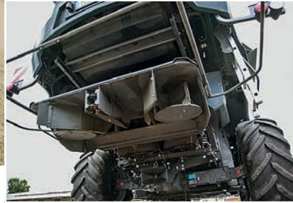
After a tweak to the way in which the ActiveSpread SwingFlow was installed, chopped straw was distributed evenly.
