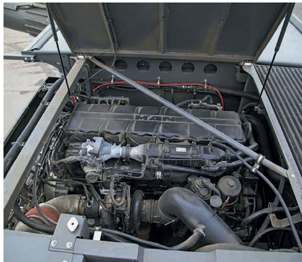
The MAN engine delivers up to 647hp; the radiator sucks in air from above, and, thanks to the reversible fan, it rarely needs blowing out. This helps to minimise daily maintenance time.
