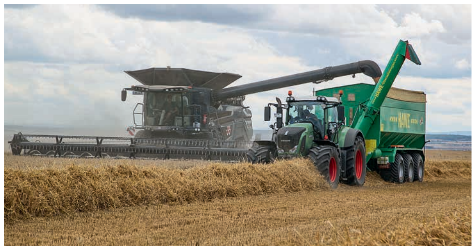
A 4.4m unloading height is a bit low and the tube length doesn't match the 10.70m cutting width. By comparison, the 17m 3 grain tank and emptying rate of 80 seconds are benchmark setters.
