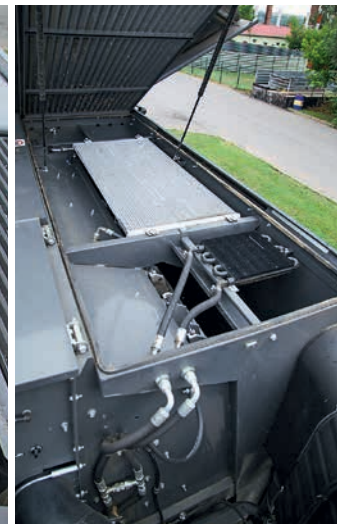
The MAN engine delivers up to 647hp; the radiator sucks in air from above, and, thanks to the reversible fan, it rarely needs blowing out. This helps to minimise daily maintenance time.
