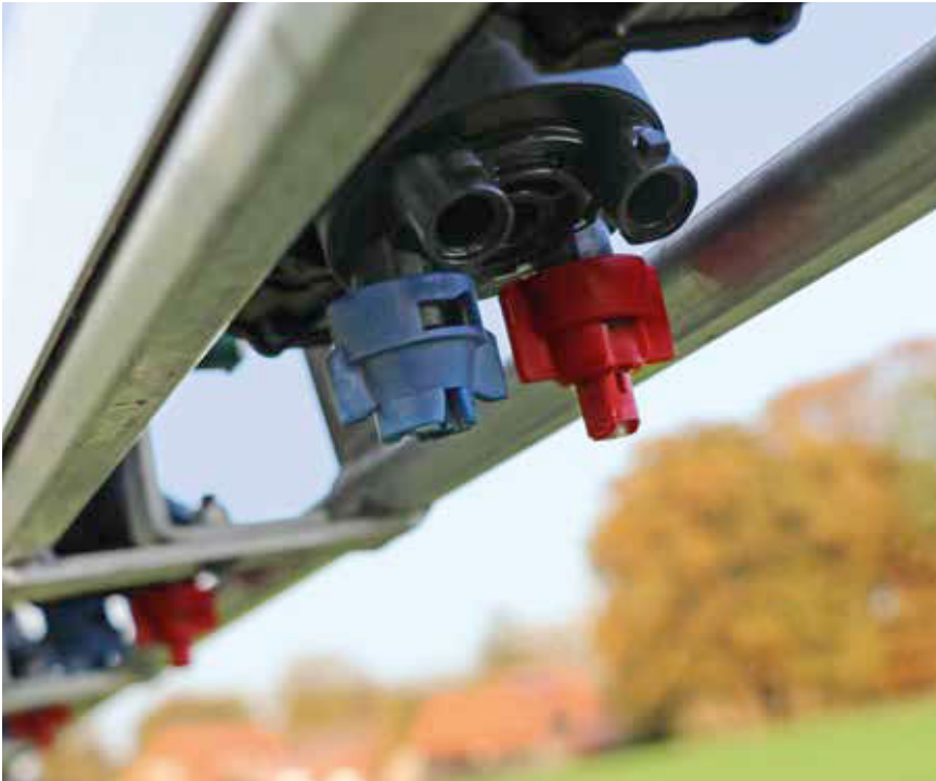
In combination with Fendt OptiNozzle, the sprayer and tractor work together efficiently. The crop protection sprayer calculates the optimum speed to match the nozzle parameters, the desired drift reduction and application rate.
