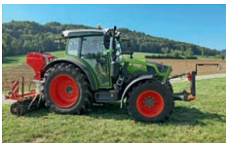
The Fendt tractor is equipped with a camera that identifies the bare spots in the stand.
