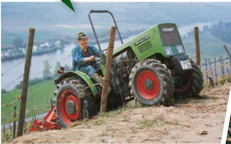
▲ The Fendt Farmer 200 V reached 25 km/h in fast speed mode and was specially developed for sideline farmers and specialist crop farms.
