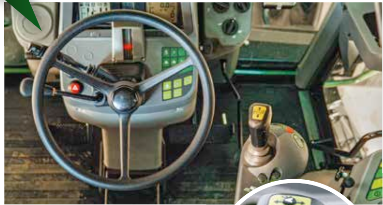
► The first-generation joystick made it much easier to operate the tractor.
