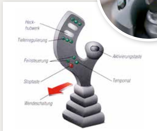
► The first-generation joystick made it much easier to operate the tractor.
