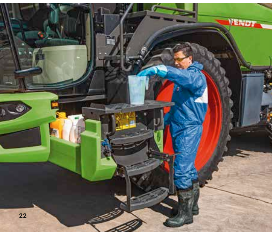
◀ It is extremely easy to fill the Rogator with liquid pesticides. The 60 l capacity induction hopper has an output of up to 200 l/min.
