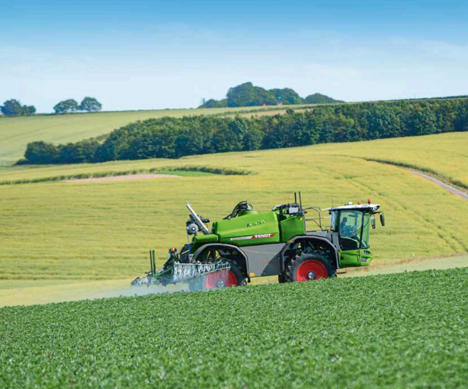
▲ The unique parallelogram suspension subtly transfers chassis movements to the 36-metre boom.
