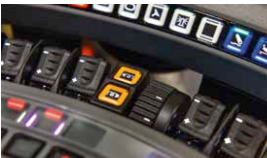
▲ With the IOM (Individual Operation Manager) you can reassign most buttons to different functions.
