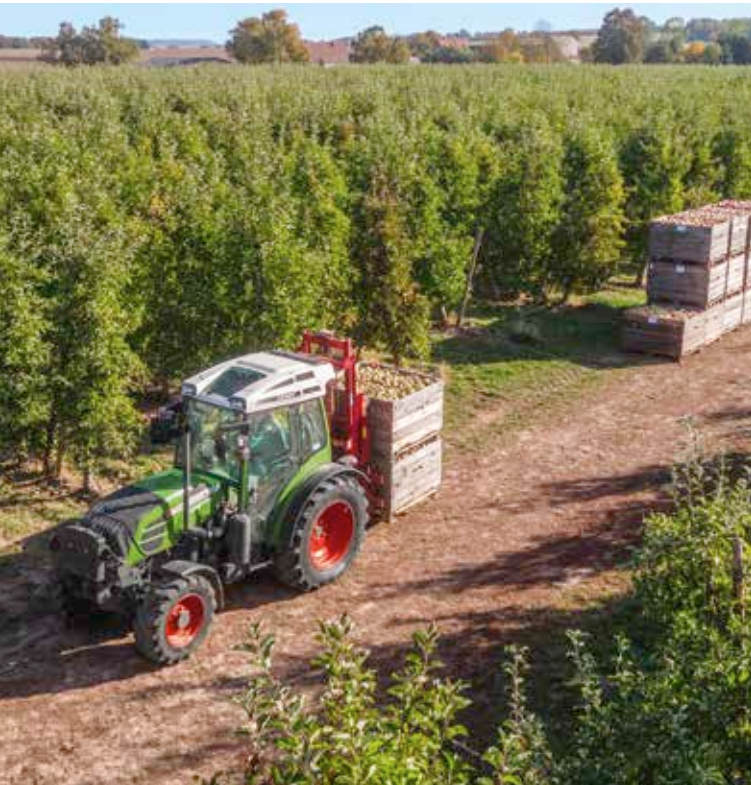
▲ Advantage of the swinging power lift – precise alignment of the implements and precise control of the rear lift truck.
