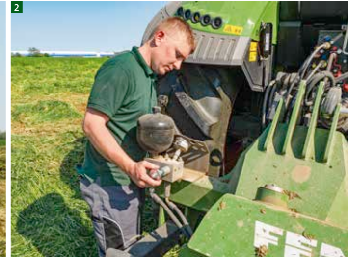
2 Fendt grassland expert Johannes Grötsch adjusts the contact pressure of the Fendt Slicer 3670 TLXKC disc mower via the hydropneumatic TurboLift system. The grass sward is protected by the floating cut which produces optimal forage quality. The forage always stays free of dirt even in wet and damp places.
