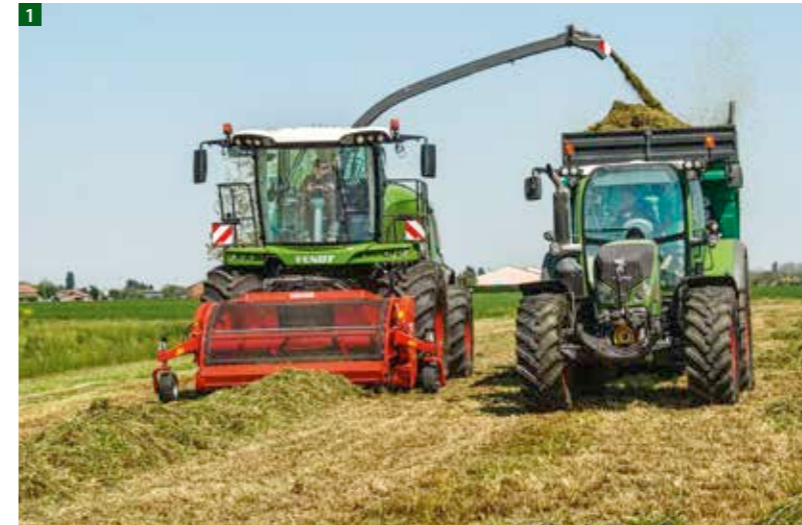
1 The Fendt Katana 85 with the Kemper P3002 grass pickup and new HD drive also achieves high output under extreme harvesting conditions. The centrally integrated gauge wheel ensures better ground following. The continuously variable header drive allows you to adjust the pickup speed to precisely match the harvesting conditions and the forage harvester's forward speed.
