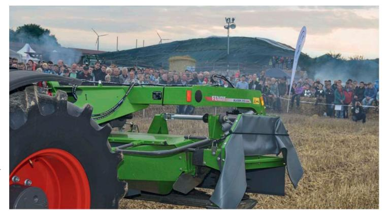
Alongside tractors and harvesters, AGCO/Fendt demonstrated the new Fendt implements in Mosheim. Here we see the Fendt Slicer mower for efficient forage harvesting.
