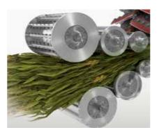
The greatest possible compression of the cut material thanks to 6 feed rollers, pre-tensioned with large-dimensioned spring assemblies.
