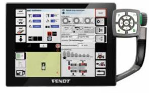
To convert engine power into forward propulsion in the best possible and most gentle way — no matter what kind of work or under what kind of conditions — the Fendt Grip Assistant quickly and easily helps you find the best ballast, the right speed or the optimal tyre pressure.
