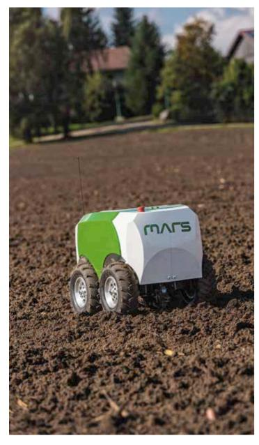
MARS robots can, for example, go out into the fields earlier in the spring to sow seeds, where larger machines would just sink into the wet soil.
