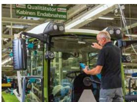
Noise protection test with the aid of ultrasound technology in the cab factory in Asbach-Bäumenheim
