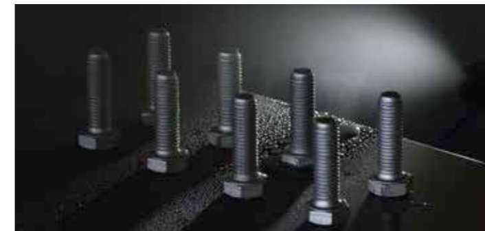
Highest standards in the details: The salt spray tests, which we use to test all the external components of the tractor for corrosion, last up to 600 hours.
