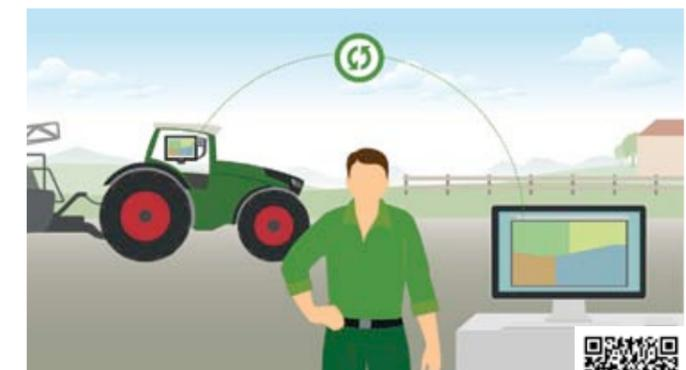
VRC: The job is transferred to the Varioterminal in the tractor either per mobile network or Bluetooth.
