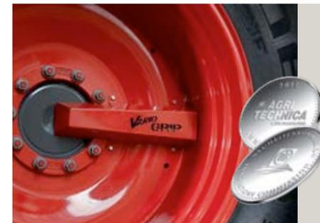
**The right tyre pressure is a topic that Fendt has been pursuing for a long time. With VarioGrip, Fendt is the only manufacturer up to now that offers a fully integrated tyre pressure regulation system directly from the factory. To assist professional farmers, contractors and machine operators, in choosing the right ballast and in setting the correct tyre pressure, Fendt has now developed a new assistance system Fendt Grip Assistant for the 1000 Vario series.**
