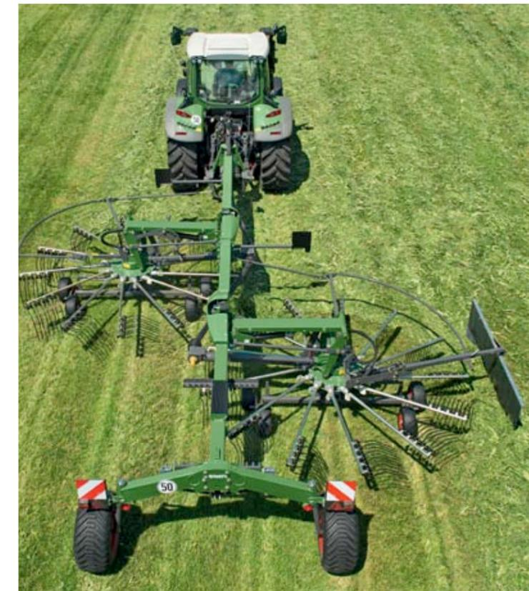
other. On the Fendt Former 12555 X, however, it is possible to adjust the speed on each rotor separately – independent of the engine and ground speed of the tractor. This makes it possible to react quickly and individually to the different structures of the forage crop.
