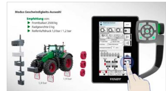
Adapted ballasting and correct tyre pressure are decisive variables in minimising power loss due to slip and rolling resistance.
