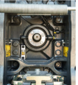
Select between two PTO speeds: 1000 and 1000E.
