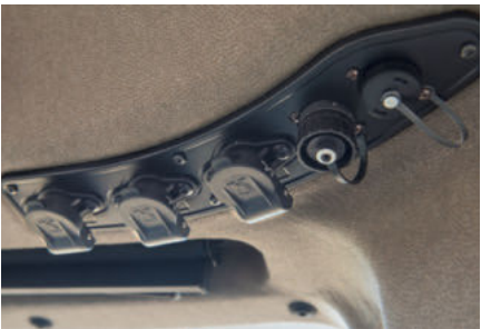
Power connections for external consumers are tidily arranged and can be easily accessed in the roof area.
