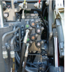
The hydraulic system is designed for maximum performance and offers the option of up to 440 l/min performance at 1,700 rpm.
