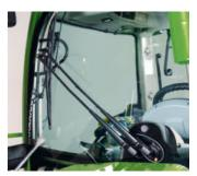
Two windscreen wipers to choose from: Segment wipers with intermittent operation or parallel wipers for an even larger wiper field.
