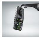
The wide-angle mirror is integrated as a second mirror in the housing, providing excellent visibility for turning and avoiding blind spots. The second variant is the electrically adjustable heated rear-view mirror (Profi/Profi+).
