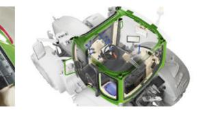
The clever ventilation and air-con design distributes the air perfectly from the steering column and from a side vent for the right window. There is also an overpressure and auto defrost function. The inside temperature is displayed on the dashboard. The foldable roof hatch provides draught-free ventilation.
