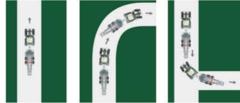
Automatic steering axle lock: This assist system unlocks the trailer's self-steering axle at a predefined speed. On straight stretches, the locked self-steering axle ensures stable handling. Operators do not need to lock the self-steering axle manually outside of the preselected speed range or when reversing.
