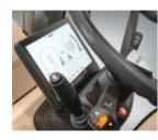
Central dashboard With its modular design, the Fendt 300 Vario can be perfectly adapted to your requirements with a range of equipment to choose from. The Power variant starts with the high-performance, adjustable 10" digital dashboard. Simply adjust the settings with the new pushdial on the righthand armrest. The entire cockpit can be completely rotated and adjusted by foot pedal.
