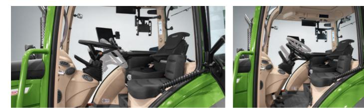
Perfect ergonomic adjustment: The steering wheel and cockpit are easy and quick to adjust with the foot pedal. For the best sitting position, the steering wheel and cockpit must be at the right height and tilt angle. Benefit: The best view and minimal glare in the cockpit. For a comfortable exit, just pivot the steering column and cockpit upwards with the foot pedal.
