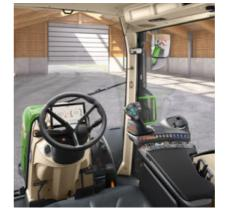
**Power Setting 1** - No crossgate lever - 1 linear module (rocker pair) to control hydraulic valves
