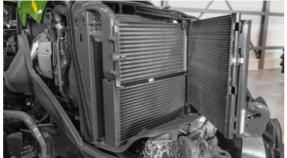
Less effort: The compact radiator package is very accessible and can be cleaned easily and quickly because of the generous clearance between the coolers and the flat radiator bottom.
