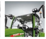
$\hfill\square$  Variant with fold-out panoramic window and door on the right. Includes an additional second handle to close the window. This ensures the window is very secure and fully sealed when closed, and keeps the noise out.
