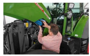
The high-performance air filter achieves optimum air intake and cleaning and is easy to replace.
