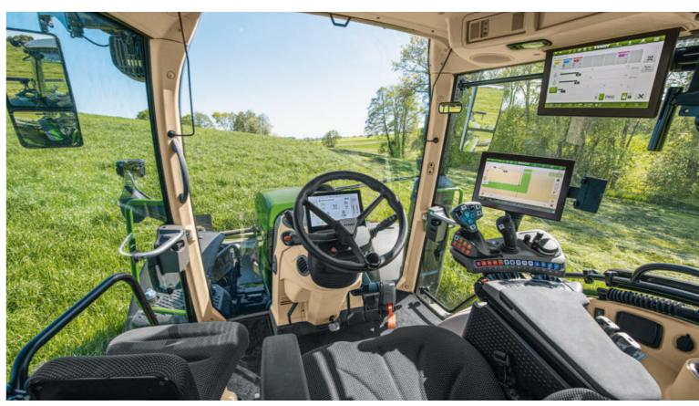
Fendt offers a clever solution for cables that run from the rear of the tractor into the cab. Cables can be guided through the lead-through, no matter what kind of cross section they have. The rear window can be closed, so dust, dirt, water and noise stay outside.
