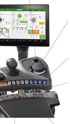
Use the central pushdial to decide what to display on the Fendt 300 Vario. This includes four quick access keys for Back, Launchpad, Overview, Individual Operation Manager (IOM) and switching between terminal and dashboard.
