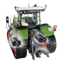
2,690 kg: 64 weights on the inside and outside of the undercarriage (32x per tread)
