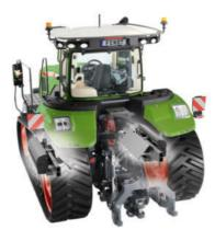
1,345 kg: 32 weights on the outside of the undercarriage (16x per tread); dirt guard on the inside
