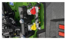
Assembly – Options • Compressed air brake system
