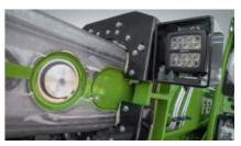
Dirt scraper • Prevents dirt from entering the interior of the telescopic boom and damage occurring
