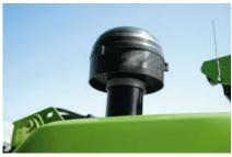
• Cyclone pre-separator for the air filter (up to 98% separation)
