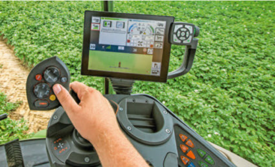
The Varioterminal 10.4" provides the perfect overview of your Rogator 600 with SectionControl, VariableRateControl and VarioDoc Pro. The Rogator 600 multifunction joystick puts all functions within easy reach.
