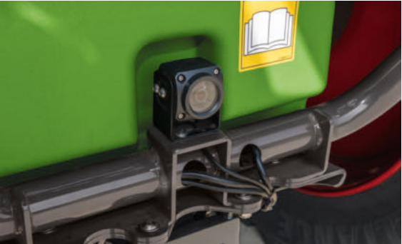
The optional camera provides with the ideal view over the area behind the machine.
