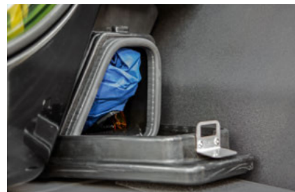
• Storage compartment for gloves and protective clothing • Keeps PPE out of the Cat 4-certified cab
