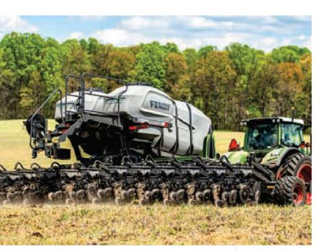
**In-line tandems** not only eliminate pinch rows, but the patent-pending transport carriage system is also an integral part of Momentum's weight management and inflation systems.
