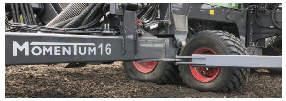
The automatic tire inflation is part of the Load Logic compaction management system. The Smart Spindles measure the weight being carried on Momentum's tires and the algorithm automatically set optimal tire pressures.
