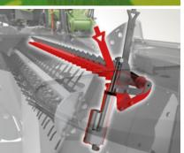
Electric motor steplessly controls the counter comb of the conditioner, which is responsible for the intensity of the conditioning process
