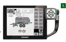
Parallel operation via control lever transfer, Varioterminal and Tigo -Terminal (option)
