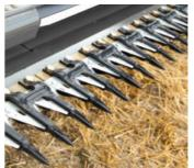
The FreeFlow table has feed fingers over the entire width, which increase the throughput of the intake auger and guarantee active, fast feed into the crop elevator.
