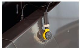
The returns camera can be used to track the threshing quality at all times, and to react quickly and easily to the changing harvest conditions.
