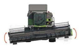
The standard AutoLevel table control ensures a constant cutting height over the entire width.
