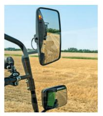
A clear view to the table and stubble, and to the spreading pattern of the straw chopper with the camera, enables the best performance in the field.
