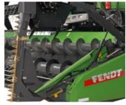
The optional rapeseed auger increases the crop flow to the crop elevator in high crops and enables an increased throughput rate.
