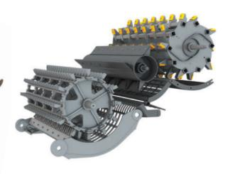
To minimise material wear caused by dirt entering the machine, we use very low-wearing materials in our rice combine version – especially for the machine components that come in direct contact with the crop.
