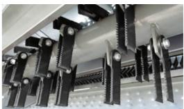
Electrically adjustable deflector plates are also available as an option. The distribution can always be best set from the cab.
