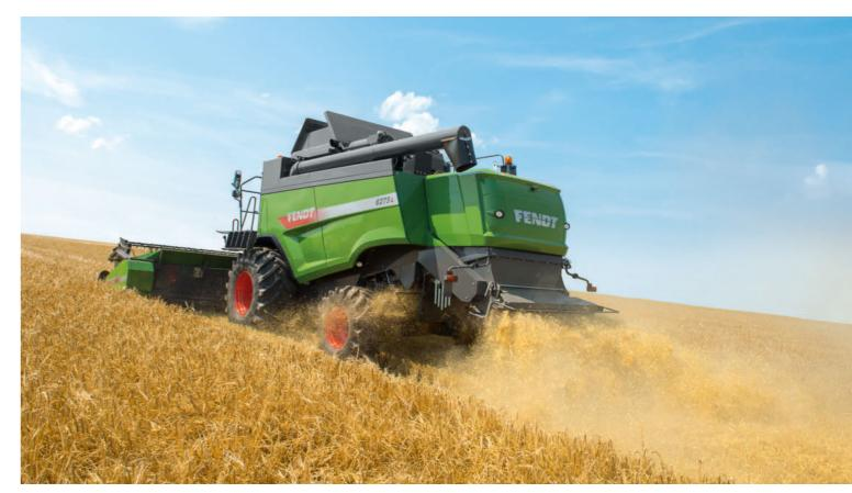
Operators can switch quickly and easily between swathing and chopping modes, simply by moving a lever.
