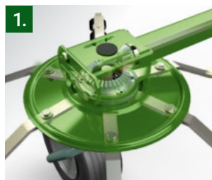
1. Induction-hardened and ground tooth flanks ensure smooth running and high break resistance
