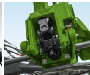
Stable drive train consisting of hexagonal shaft and double universal joints
