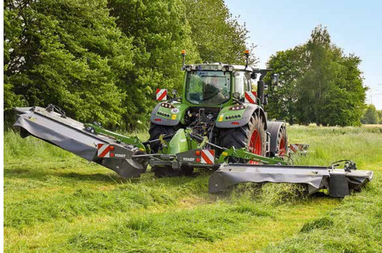
△ The rear-mounted mowers also lift out individually when cutting awkward areas. The function can be preselected on an electronic box.
