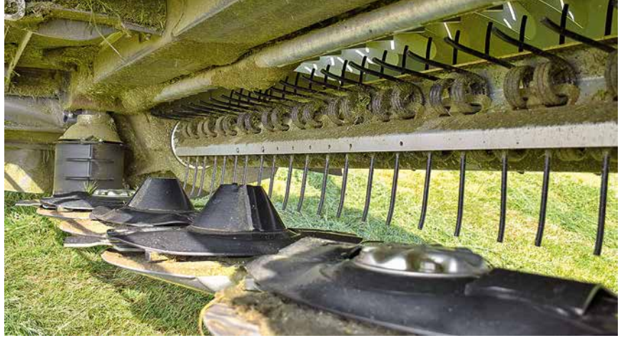
△ The spring tines on the conditioner pull the material through an adjustable comb.
