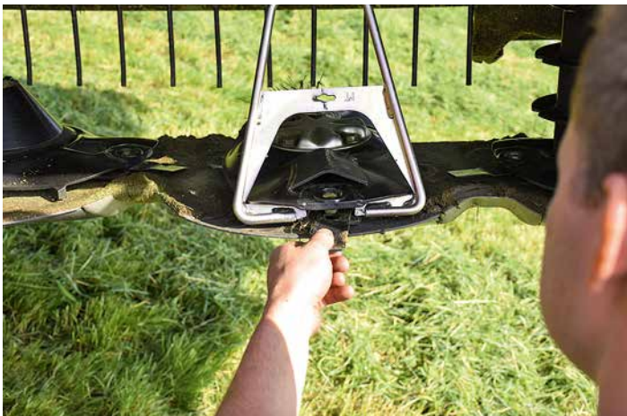
△ The rear-mounted mowers also lift out individually when cutting awkward areas. The function can be preselected on an electronic box.
