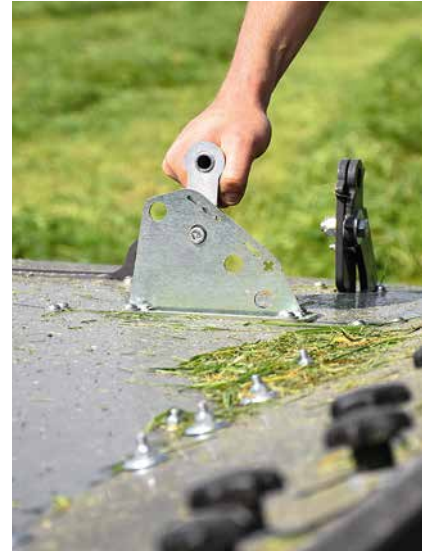
△ This mechanism adjusts the comb to one of four positions.
